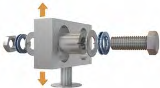
Fig 2: Drawing of the test rig. The assembled parts are vibrated vertically and the joints are subjected to two impacts per cycle. The impacts are parallel to the bolt. The arrow displays the direction of vibration during the test. After testing, the fasteners are inspected for rotation.
